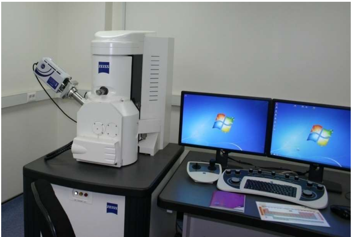
4.2.1-rasm. Skanerlovchi elektron mikroskop — SEM EVO MA 10 (Carl Zeiss)
